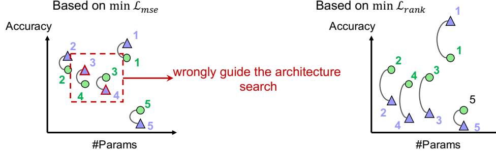
Fig. 2: Considering five pairs of the true (green circles) and predicted (purple triangles) values. An MSE loss aims to minimize the Euclidean distance between the true and predicted values (i.e., left sub-figure). While a ranking-based loss aims to maintain the same ranking between sorting based on the true and predicted values (right sub-figure). For the purpose of differentiating architectures during an EA process, a high-rank correlation is required, while a low MSE is desirable but not required.
