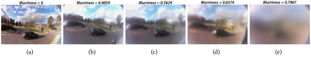
Fig. 3. Effects of using blurry filters. (a) The original image. (b) Using one frosted filter with translucent tape. (c) Using two frosted filters with translucent tape. (d) Using three frosted filters with translucent tape. (e) Using one frosted filter without translucent tape.
