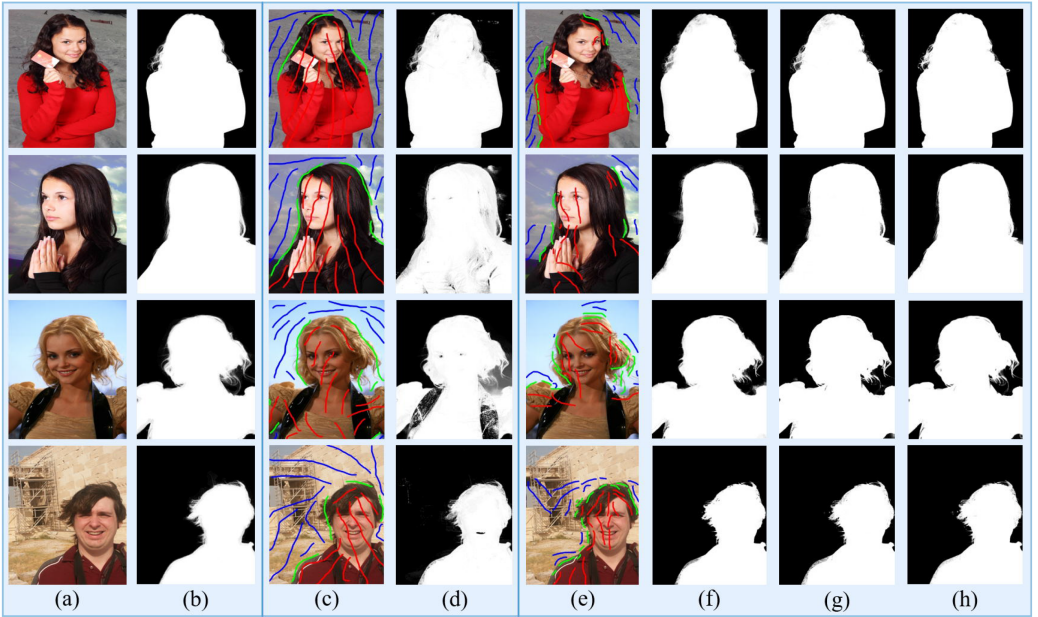
Fig. 6. The visual comparisons with traditional scribbles. (a) The input images from the portrait testing dataset or the DIM [38] dataset. (b) Ground truths. (c) Traditional scribbles. (d) Traditional scribbles + DCNN [8]. (e) Smart scribbles . (f) Smart scribbles + KNN [7]. (g) Smart scribbles + DCNN [8]. (h) Smart scribbles + IFM [2]. The alpha mattes produced by smart scribbles have more complete outlines and abundant texture details.
