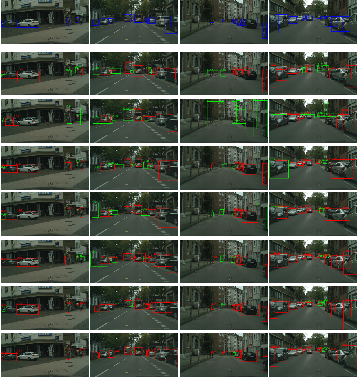
Fig. 12. Qualitative results of the proposed method on the Cityscapes dataset. The first row shows the GT bounding boxes in blue. The other rows show the results of different methods when 1000 top ranked proposals are used. From top to bottom: BING [2], Objectness [1], Selective Search [6], Edge Boxes (Edge 50) [11], MCG (Accurate) [37], Faster R-CNN (VGG) [38] and our method. Red rectangles indicate corresponding instances that are successfully detected (i.e., \text{IoU} > 0.5 ), while green rectangles indicate instances that fail to be detected by any proposals. The numbers on top of each rectangle shows the IoU overlap with the instance.
