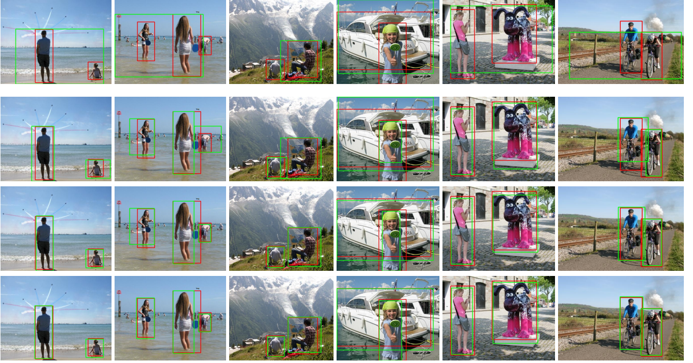
Fig. 9. Qualitative results of the proposed method on the StereoObj dataset. The ground truth bounding boxes are in red color. The corresponding best proposals are in green color, obtained from the top N proposals. From top to bottom: N = 1 , N = 10 , N = 100 and N = 1000 .
