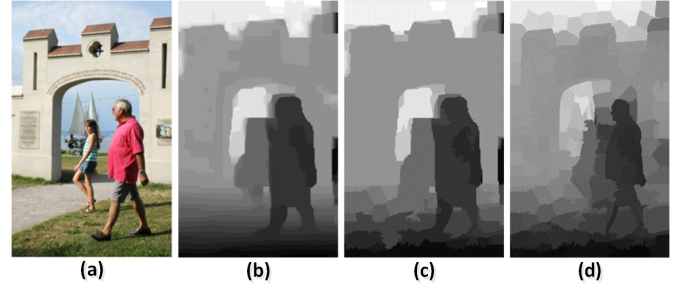
Fig. 2. Example of rough depth map enhancement. (a) Color image. (b) Rough depth map. (c) and (d) Results after enhancement with different numbers of superpixels.
