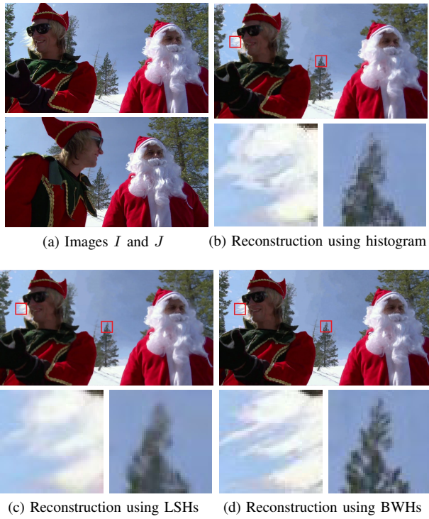
Fig. 3: Histogram matching examples. Image I is reconstructed from image J and the dense patch map from I to J . Traditional histogram in (b) is not suitable for content-aware applications. LSH in (c) obtains better matching results but still not distinct enough. The proposed BWH in (d) maintains the efficiency of histogram and achieves the best results.
