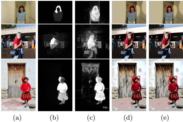
Fig. 16: Importance of detecting the entire salient objects to portrait stylization [48]. (b) The saliency maps produced by GMR [50] fail to detect faces of the salient objects. (c) The saliency maps produced by the proposed method include the whole salient objects. Hence, the stylization results of GMR [50] (d) cannot preserve face details, while the proposed method can (e).
