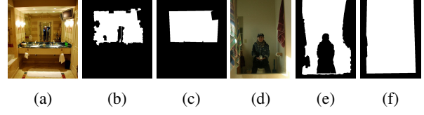
Figure 7: Two wrongly annotated examples (a) and (d) from the original datasets that form our benchmark. While the mirror masks provided by the original dataset (b) and (e) are very coarse, the regions representing the reflected persons are not considered as part of the mirror. Our corresponding ground truth masks are shown in (c) and (f), respectively.
