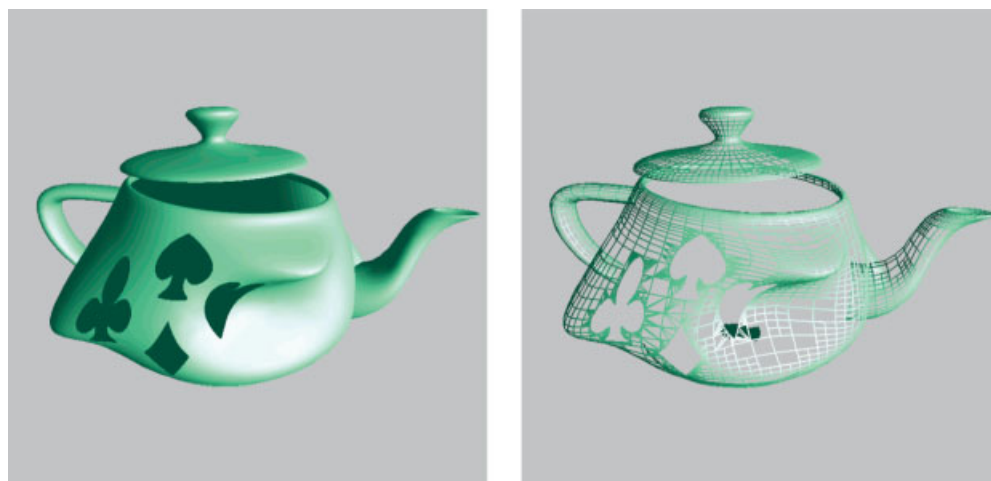
Figure 8. A teapot modelled by a trimmed NURBS surface: shaded and wireframe.
