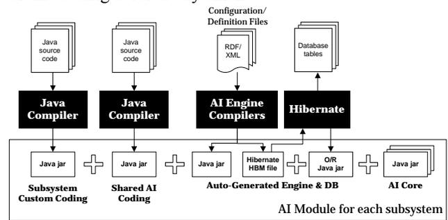
Figure 3. Software components in each subsystem’s AI Module.
