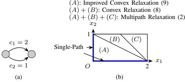
Fig. 3. (a) A simple network with one user and two links. The user can choose one link to send data from the node on the left to the node on the right. (b) Comparison among the feasible region of sparse (single-path) routing problem (1), convex relaxation (8), improved convex relaxation (9) and multipath relaxation (2) for the network in (a).
