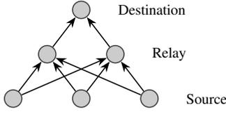
Fig. 5. A sample of relay network with three source nodes, two relay nodes and a single destination node. A user at each source node sends data to the destination node through some relay nodes.
