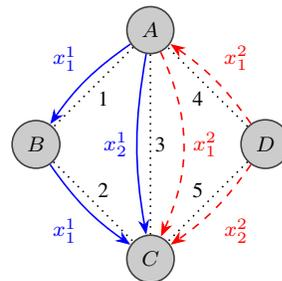
Fig. 1. A sample network with five links (dotted line) and two users. The first user, whose source is  $A$  and destination is  $C$ , has rate  $x_1^1$  and  $x_2^1$  on its two paths (solid line). The second user, whose source is  $D$  and destination is  $C$ , has rate  $x_1^2$  and  $x_2^2$  on its two paths (dashed line).
