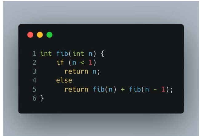
Fig. 3: C snippet that calculates the Fibonacci number, with a few errors deliberately added in.
