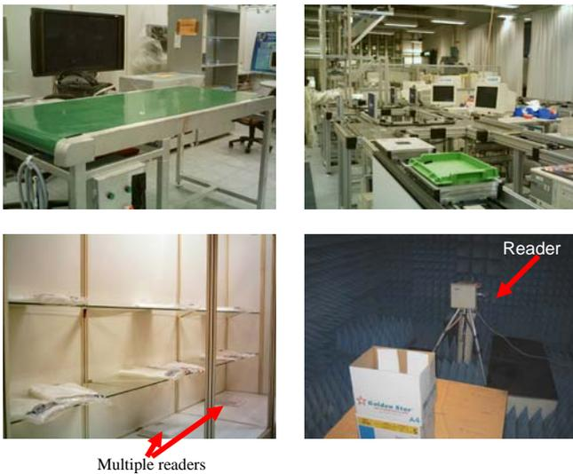
Figure 1: From upper-left and then clockwise: a conveyor belt system; a simulation system of supply chain; benchmark measurement in anechoic chamber; and a scene with multiple tags and multiple readers.
