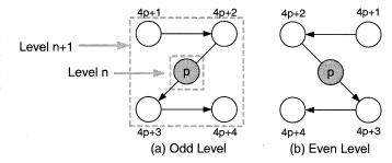
Fig. 2. Z-ordering indexing scheme.
