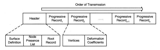
Fig. 3. Structure of a NURBS stream.
