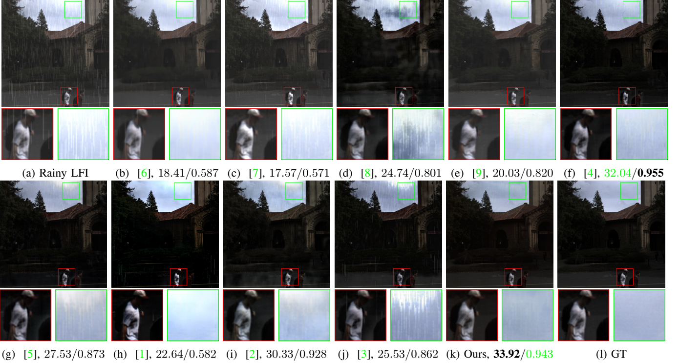
Fig. 1: Comparisons of different methods for rain streaks removal on LFI. The de-rained image of each method is marked with its PSNR/SSIM values. The best value is marked in bold , and the second best is marked in cyan.
