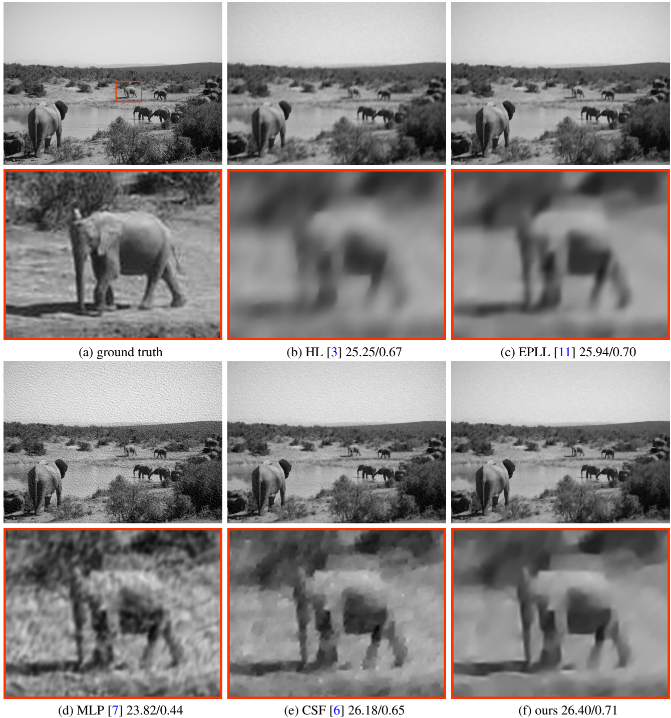
Figure 5. Comparison of different non-blind deblurring methods with ground truth kernel under 5% noise. PSNR and SSIM are shown in the figure.
