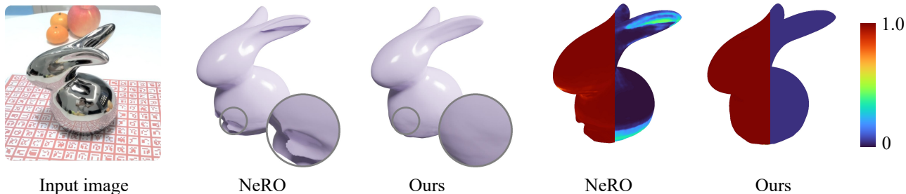
Figure 1. Inverse rendering results of the cutting-edge method, NeRO [10], and ours from calibrated multi-view images of a glossy object. Geometries are shown as a rendered mesh in the second and third images, and materials (metalness & roughness) are shown as a color map in the fourth and fifth images. We can see that our results not only have smoother and more accurate geometry but also present a more reasonable material (since the material of this object should be uniform).
