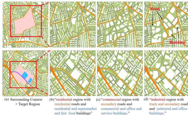
Figure 1: Text-driven Urban Layout Regeneration. Given the target region (pink region in (a)), Text2City regenerates its urban layout based on the textual layout description and the surrounding context. Orange and gray lines represent main and minor roads. White polygons represent buildings. Purple lines and blue polygons represent roads and buildings to be preserved, and are provided by the user as constraints. (b)-(d) are regenerated layouts of the red box in (a), based on different input textual layout descriptions.
