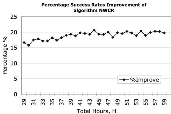
Chart 8. The percentage success rate improvement of Algorithm 3 (NWCR). Algorithm 3, on average, performs roughly 18.9% better than Algorithm 2b in successfully scheduling meetings.
