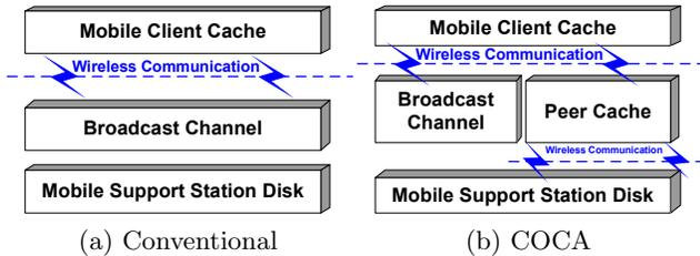
**Figure 1: Storage hierarchy of push-based mobile systems.**
